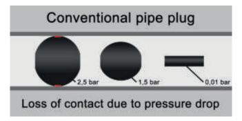
These pipe plugs contact the pipe wall only when nearly at their full working pressure. In the event of a drop in working pressure, they contract, causing them to lose contact with the pipe and be pushed away by the back pressure caused by the standing water. Clearly, such pipe plugs are very unsafe! This is the reason why expandable pipe plugs must be secured in place by bracing.
