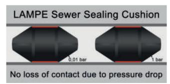
As shown above, the cushion when inflated with only 0.1 bar is already in full contact with the pipe wall. Therefore, even a significant drop from the nominal working pressure will not impair the contact with the wall. There is always enough time to control and readjust the pressure loss.
